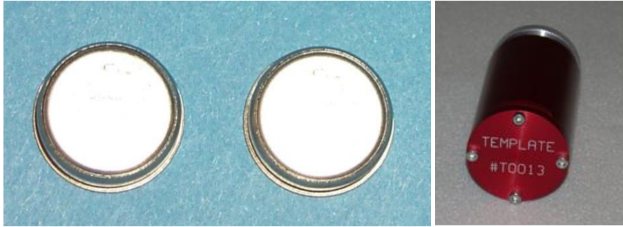
Figure 1: The memory devices used to store the TRIS template (left), and the iButton (right) which is an aluminum housing for the memory devices storing the template information. (Photo Credit: Sandia National Laboratories)
