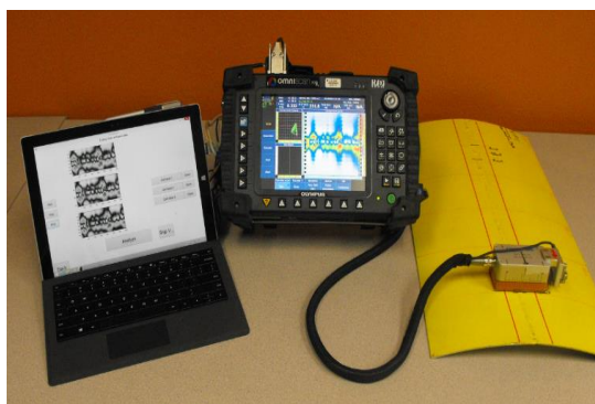
Figure 2: Eddy Current Array Probe with Calibration Specimen. (Photo Credit: Pacific Northwest National Laboratory)
