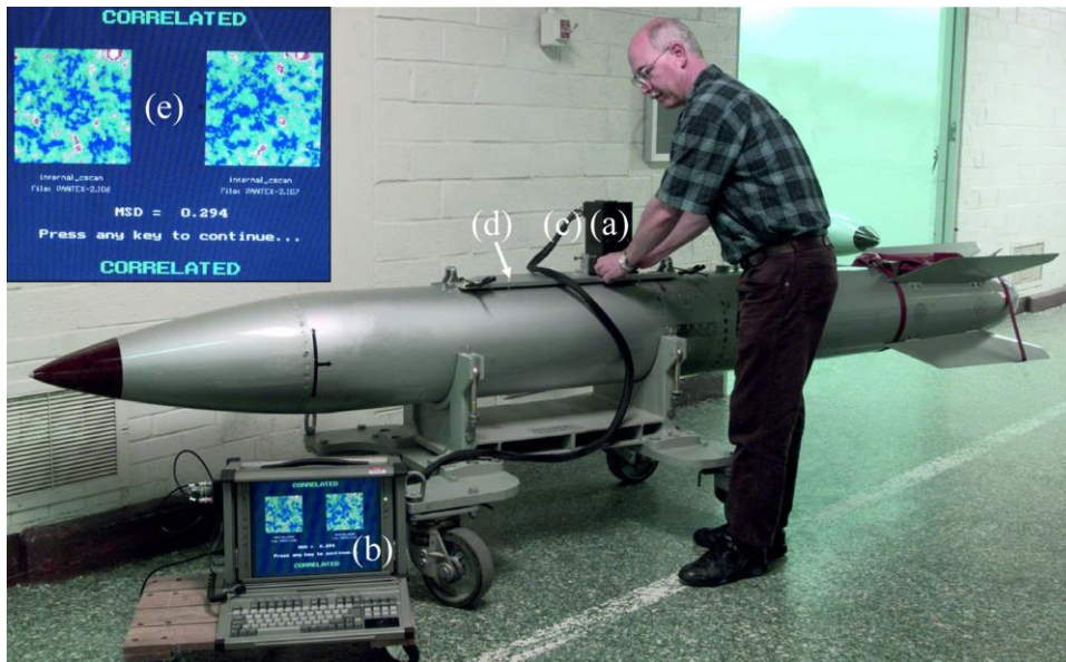
Figure 2: The UIT instrument is shown acquiring a signature from an inert Trainer. (Photo Credit: Pacific Northwest National Laboratory)
